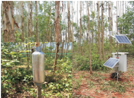
图1 试验场地布设与包裹式茎流仪安装(左下) Fig.1 Experiment site and installation for Dynagage sap flow(at the lower left)
