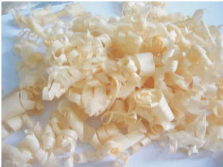
图 3 亚微米刨花加工到最薄厚度时的絮状结构 Fig. 3 The floc structure after processing to the most thin thickness of the submicron shavings
