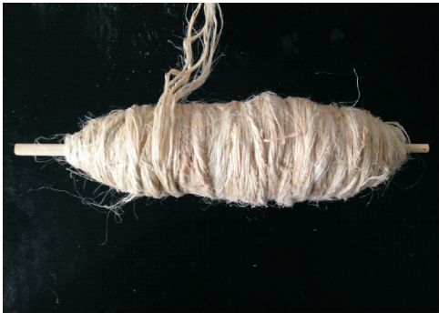
图 3 预处理后的菠萝叶纤维束 Fig. 3 Pineapple leaf fiber bundle after pretreatment
